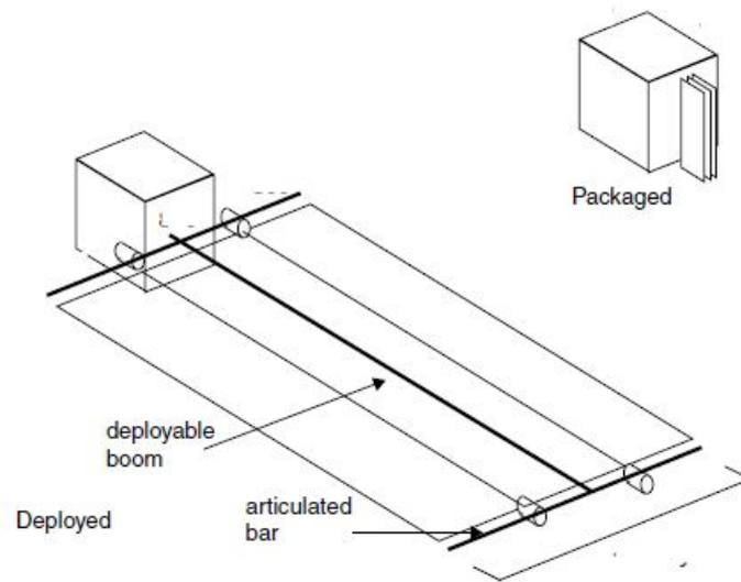
Fig. 5.10 Double fold and roll-up solar array.
