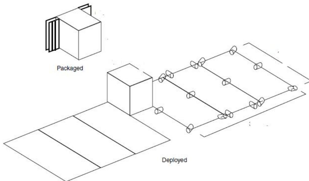
Fig. 5.12 Split Solar arrays three fold
