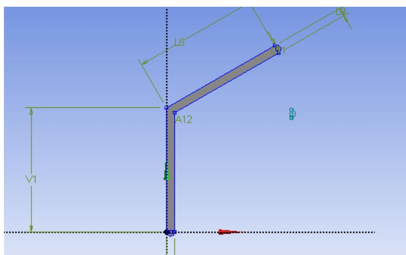
Fig. 6.7 Cross section of supporting beam( $V1 = L8 = 30\text{mm}$ ,  $A12 = 120^\circ$ )
