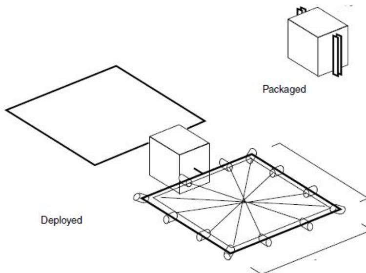
Fig. 5.11 Solar arrays that fold into two bundles of bars
