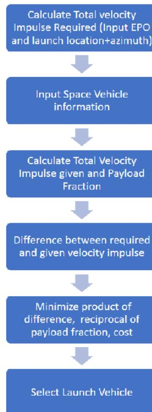
Fig. 3.2 Launch Vehicle Selection Code Flow Chart
