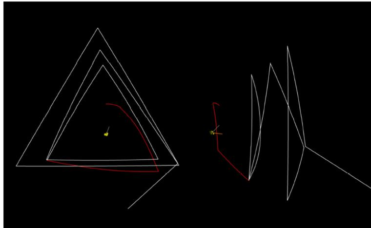
Fig. 2.4 Rendering of the triangular maneuvers around the comet
